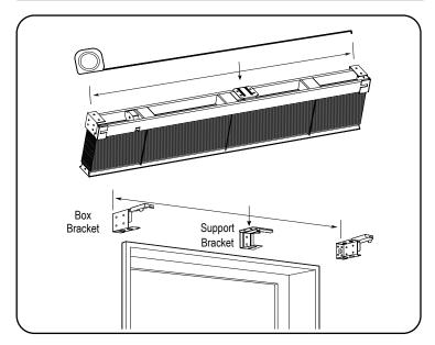
Place box brackets on headrail. Evenly space support brackets between box brackets, away from ladder cords. Using a tape measure, measure bracket locations. Mark bracket positions.
